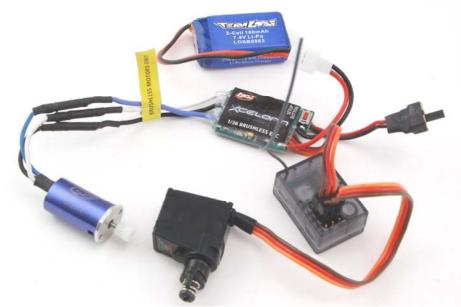
An example of connection for LOSB9594 Brushless Combo with the motor and battery connected.
