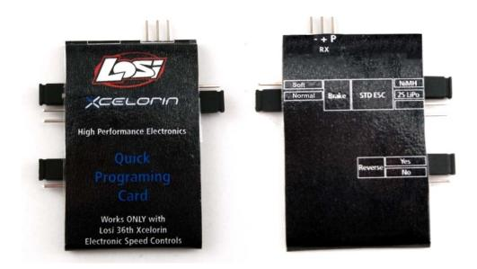
The supplied Quick Programming Card (QPC) is used to setup the Electronic Speed Control to your operating requirements.
