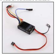
LOSB9501 Xcelorin Electronic Speed Control v1.0
