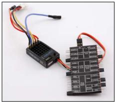
The Xcelorin Quick Programming Card (QPC) is used to make all adjustments to the active profile in your ESC. Any ACTIVE profile can be modified.
