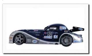
The unusual shapes of this curious endurance track GT mean that ingenuity was called for in both the front and the back. A flat, highly flexible and very low-slung chassis was chosen, and the designers managed to fit to this the pivoting motor bed of the two-wheel drive **SCX**® cars. The front wheel assembly and guide were also resolved in a feat of engineering, making use of a perfectly-fitted semi-axle.
