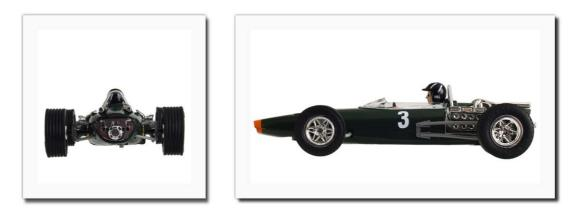
A simple chassis, the minimum for the car to move on, with measurements stretched as far as possible in terms of both guide length and axle width, gives the impression that this was a good design which took advantage of every bit of the small space available.
