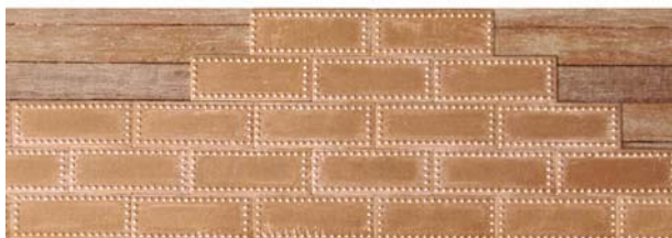
Start flush with keel and work up with 50% offsets per row
