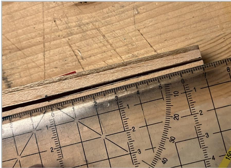
On the underside of the fuselage, the slot for the tail frame S8 is now made in the tail area, at the rear, to a length of approx. 7 cm.
