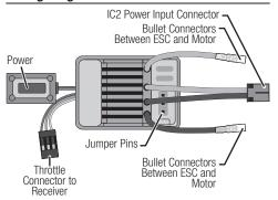
**NOTICE:** Always disconnect the battery from the ESC when you have finished operating your vehicle. If you leave the battery connected with the power switch in the OFF position, the ESC will continue to draw current when connected to the battery, resulting in possible damage to the battery through over-discharge.
