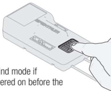
3. Release the bind button once the orange LED starts to flash continuously, indicating the receiver is in bind mode.
