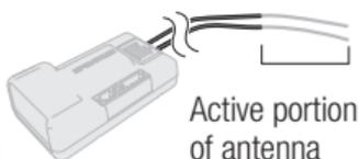
**NOTICE:** Do not cut, kink, or modify the antennas. Damage to the coaxial portion of an antenna will reduce the performance of the antenna. Shortening or cutting off the 31mm tip will reduce the range.
