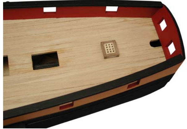
Fig 004 – Middle Hatch Assembly
