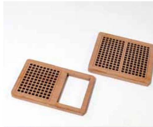
43. When dry, remove the laser char from the edges and interior ladder hatch.
