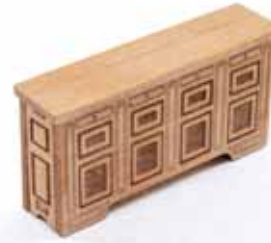
437. Glue CF-5 to the top of the cabinet, making sure that the rear edge is flush with CF-2.
