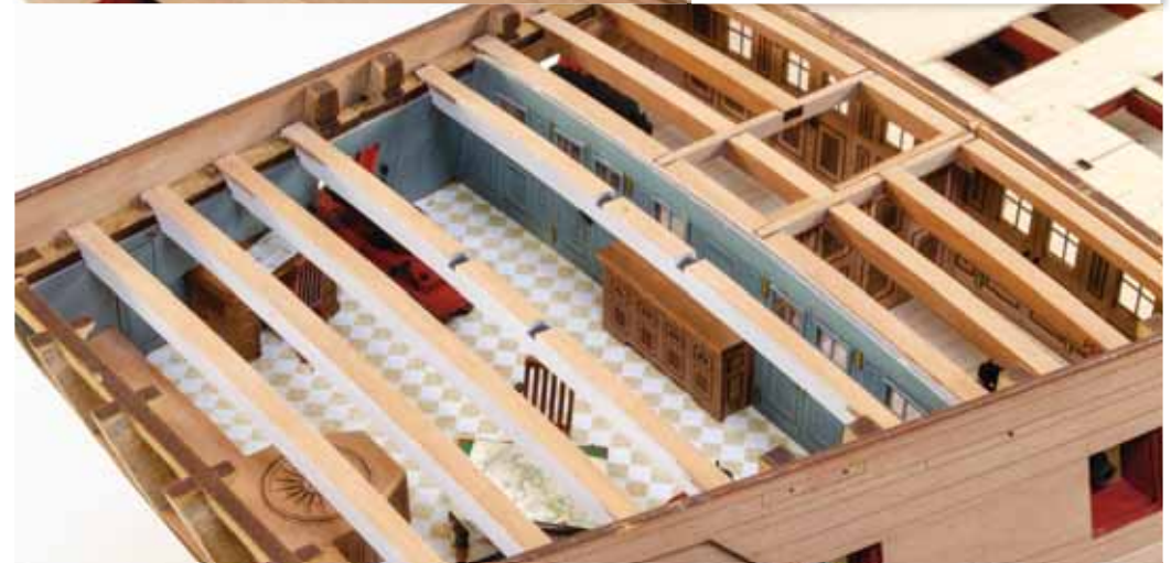
458. We can now move to the rear cabin and begin to install the deck beams there. Glue deck beams PD5, PD7, PD8, PD9, and PD10 into place.
