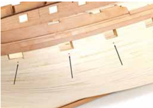
216. Referring to plan sheet which shows the main wale installation, make a pencil mark below the middle of each gun port, using the measurements on that plan. Make these as accurate as you can.
