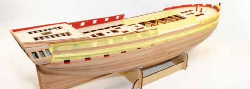
527. Using your plans for reference, glue a 3mm strip to the hull, followed by a 4mm strip directly underneath it. The 3mm strip top edge will mostly follow the upper engraved line still seen on the bulwarks, covering the channel position that you transposed earlier. This photo shows those in place and the outer area masked off so the strips can be sanded smooth.
