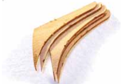
621. Leave the parts for 24hrs to dry in the jig. Remove from the jig and carefully glue the laminations together.
