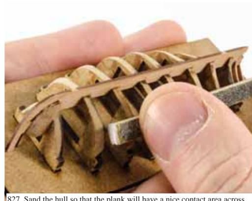
827. Sand the hull so that the plank will have a nice contact area across the whole hull.
