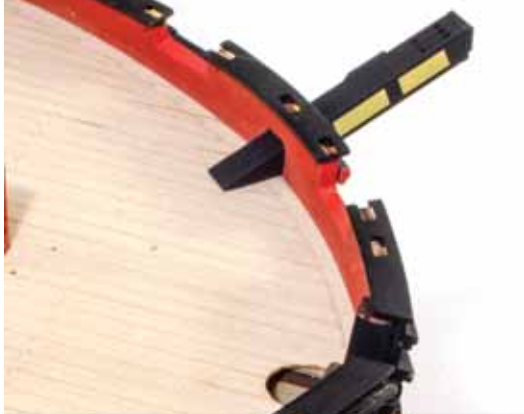
601. Glue the catheads into position, noting the side on which the cleats are fitted. These should be to the rear of the cathead.
