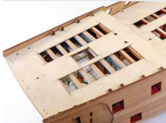
463 Carefully glue this in position, locating it into the slots in the bulkhead ears. Ensure that you don't get any glue on the open deck beam cutaways.
