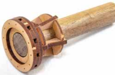
739. Use the disc to help centralise part #163 into place.
