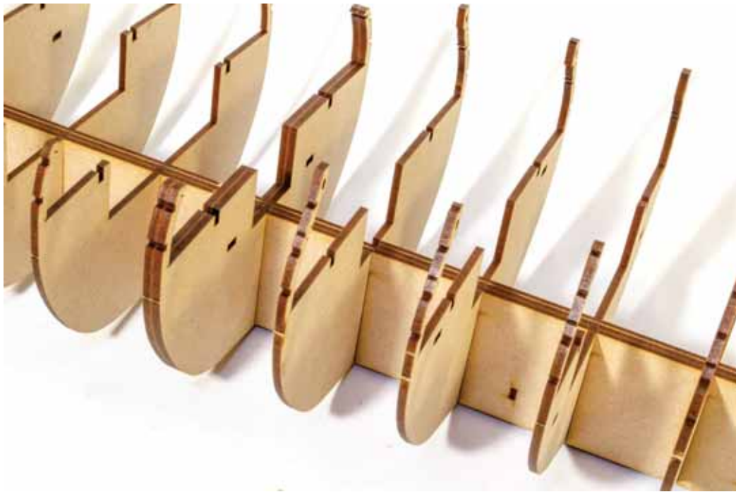
22. Glue pegs K-1 through the keel to lock bulkheads #15 and #16 permanently. You can now remove bulkhead #17 until a little later.
