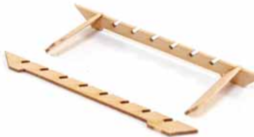
275. Glue a step into the top and bottom slots of a side piece. Leave to dry.
