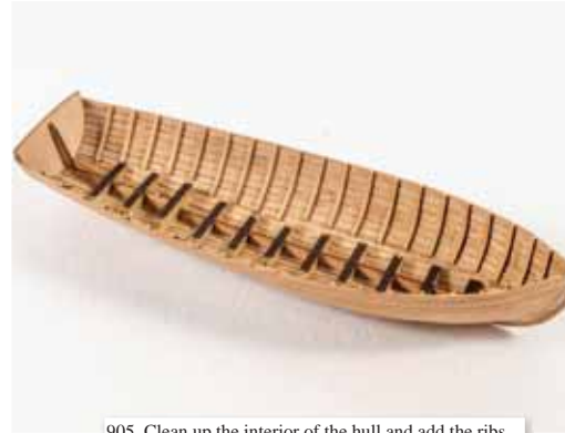
905. Clean up the interior of the hull and add the ribs.
