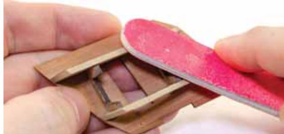
186. Take the quarter gallery frame and sand between the two protruding MDF frames, creating a sweep that angles downwards.
