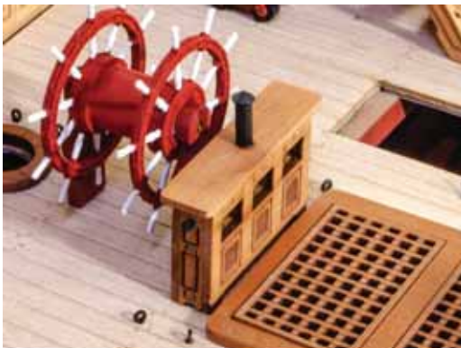
783. The binnacle can now be glued into place as shown. Lash this down to the adjacent eyebolts using either 0.5mm natural thread (not shown here).
