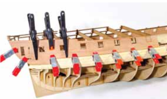
153. When the planks are dry, remove the pear bulwark sections and then use a razor saw to roughly open-up the gun ports. These will be trimmed closer a little later.
