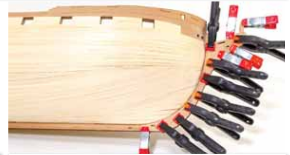
204. Take part #435 and glue/peg into position as shown. Use lots of clamps to ensure full contact with no curling. Leave until dry, then glue/clamp part #436 to the opposite side.
