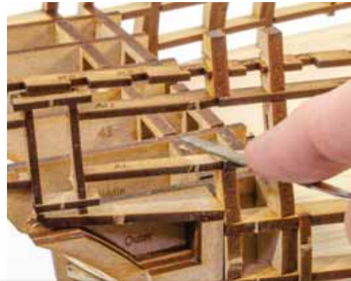
121. Carefully saw out this specific part of bulkhead #18 and file the area smooth. Also note that you can also saw and file away the parts of the strips that pass through the quarter gallery doorways.
