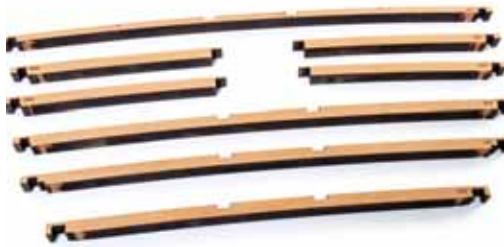
386. From the 6mm wood sheet, remove the beams for the upper deck, UD2 thru UD7. Paint the beams as you did with the quarterdeck ones.
