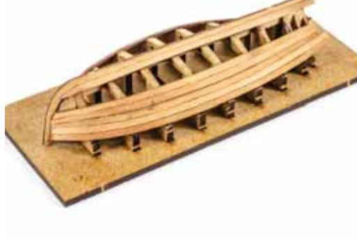
829. Taper the planks as you install, and if they become awkward to plank, then work downwards from the keel.
