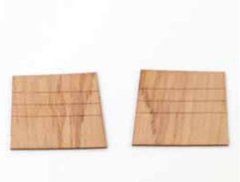
133. We have included two optional pieces (#268F) which can be used to block off the inner bulwark framing at the bow area. These are optional as they really won't be seen.
