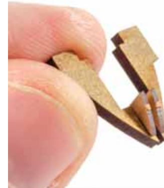
853. This boat differs slightly in that the first bulkhead has the bow timbers P15 added to it before plugging into the jig base.
