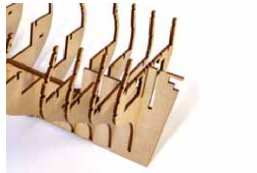
19. These can now be slotted into the keel. Again, do NOT glue.
