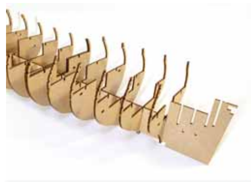
12. Now slot these into their respective slots on the keel. Again, do NOT glue.
