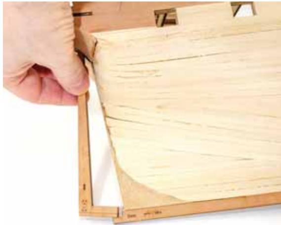
201. From the 1mm wood sheet, remove parts #437 and #438. These parts are engraved, with the narrower strip being at the bottom. Glue part #437 to the forward side of the keel. You will see this is slightly wider at the bow side.
