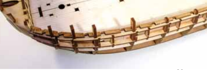
136. Fit (NO GLUE!) these strips into the bulk car slots running from bulkhead #2 thru to #9.
