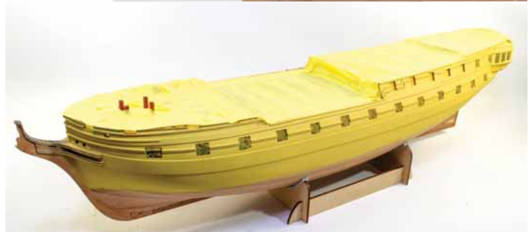
566. After carefully masking the hull and blanking any openings, paint the hull in yellow ochre. If you comprehensively mask any openings, you can airbrush this colour. Foam is used to stop paint getting into the gun ports. Note that all of the area to be painted is now in ochre. The reason is that the lighter paint makes it easy to see any defects in the hull at this stage. Paint using thin coats, run back and fill as necessary.
