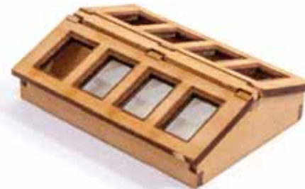
720. Glue the skylight roof panels into position.
