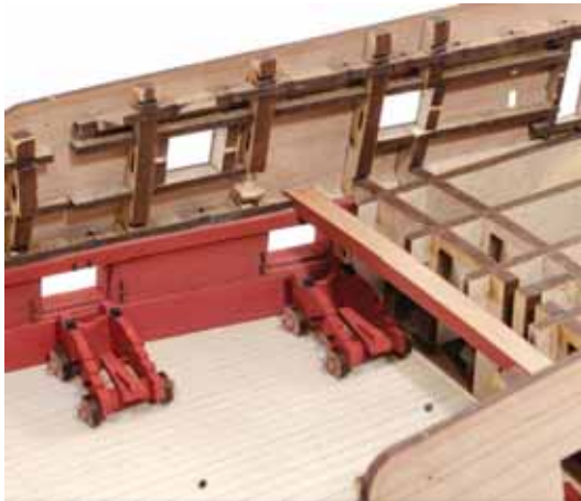
359. Remove all the char from the upper beam surfaces and then mask/paint the red, leaving the upper surface (and joint slots) unpainted. Start to fit the beams starting with the rearmost one first. NOTE: it is perfectly fine to selectively cut into and remove sections of the MDF frame so the beam can be manoeuvred into position. You can see my cuts in the photographs.
