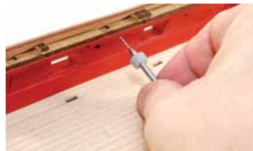
243. Use a 0.8mm or 1mm drill bit to drill through the holes in the upper ledge. This is just to make sure that if there's any tiny misalignment, that the eyelets will still fit later. Also drill through the hole positions on the inner bulwark/upper ledge, through to the outside, using a 1mm drill. This is for part of the rigging process. These holes are around the area where you will fit the cleats in the next two stages.
