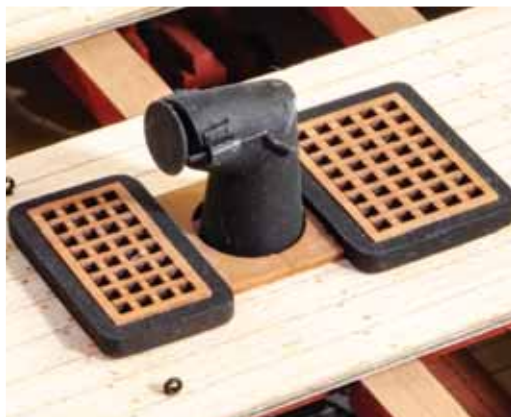
796. Paint the frames in black and glue the gratings into them. The finished assemblies can now be fitted to the deck, on either side of the stove funnel.
