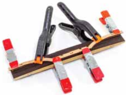
371. Lastly, glue part #306 over the assembly. Clamp and leave until dry. When the glue has set, remove the beam from the jig and clean up the outer faces so they are smooth.
