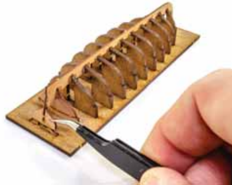
921. Glue the keel into place and also CTF-12.
