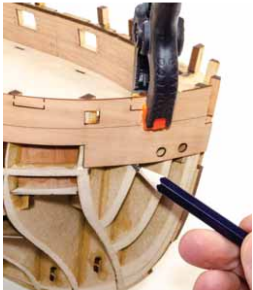
147. Draw around the bottom fore area onto the bow section, as shown. Then draw on the vertical, which should lie over bulkhead #1.
