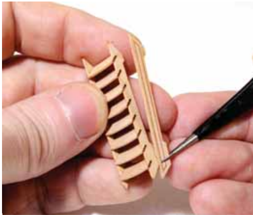
49. Now glue the side facing parts onto each side of the ladder.
