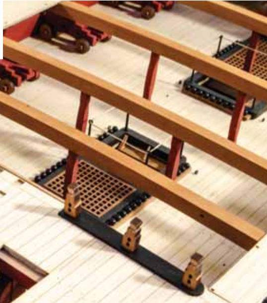
683. From the 1mm wood sheet, remove parts #301, #302, #303, and #304. From the 0.6mm wood sheet, remove parts #499 and #500.
