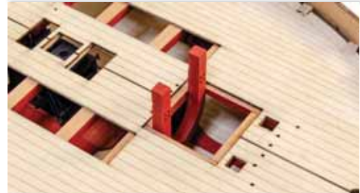
492. Insert part #187 as shown, making sure it fully locates into the deck below.
