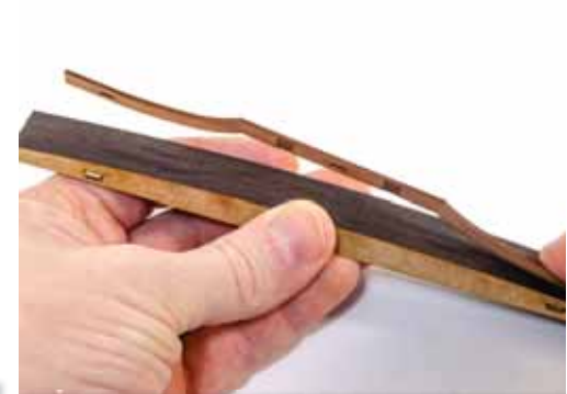
368. Lay part #168 over the jig, with the engraved side downwards.
