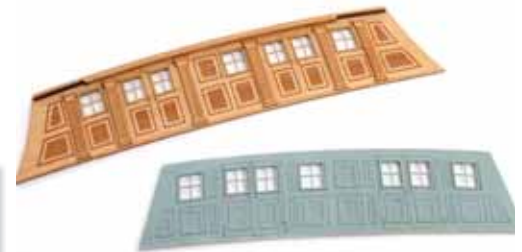
428. The window frames now need to be fitted to the windowpanes. These are found on the 0.4mm PE sheet. Please use your plans for part number against windowpane. Again, we fixed these by running clear varnish underneath the part where it sits onto the clear pane.
