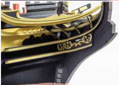
631. Now is a good opportunity to take the 0.6mm PolyBak sheet and paint all of the ornamentation in yellow ochre. From that sheet, remove parts PB-1 and PB-2 and glue either side of the bow as seen here. CA gel is ideal for this, in small spots as it allows a few seconds to finalise the position.
