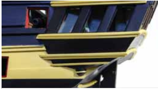
637. ...and fit them below the quarter gallery areas. The base of these is generic, so you will probably need to trim/sand them to fit precisely. TIP: If you struggle to shape the base, clip the material away below the nipple, down to base height and then glue the nipple into position and build up the base using an epoxy putty. Paint the area as shown and then add an ochre-painted rail above it. These parts are #512, found on the 0.6mm wood sheet.
