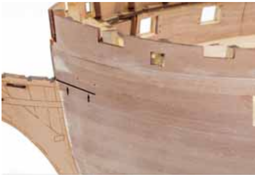
221. This is a close up showing the position of that first plank you added, as this is where the wales will now be started.
