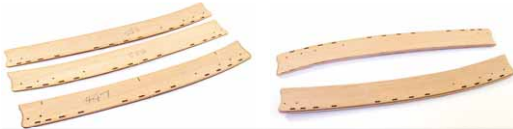
661. From the 0.8mm wood sheet, remove centre core parts #450 and #451. From the 0.6mm wood sheet, remove all outer panels #558. Round the outer edges of the inner core parts, and then round one side of the outer panels that sit onto the cores. Glue together as shown. Clamp as necessary.
