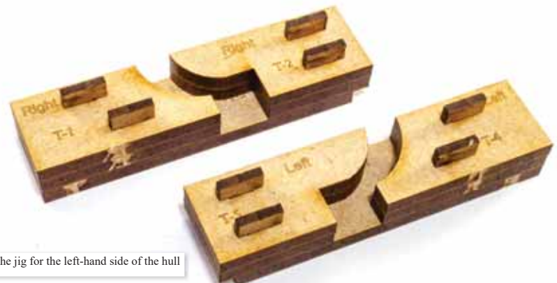
617. Glue parts T-1 and T-1 Right together, and then glue to T-3, using the pegs to align. Now glue parts T-2/T-2 Right together and glue in the pins to align. IMPORTANT. Wait for the last parts to dry before installing to the base of the jig T-3. DO NOT glue into position. This side of the jig must be able to slide.
