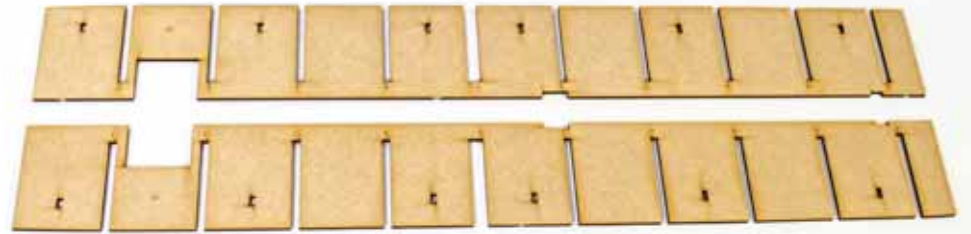
13. From the 3mm MDF sheets, remove both parts #36. Note how the slots in these are numbered. These refer to the individual bulkheads over which each slot will fit.
