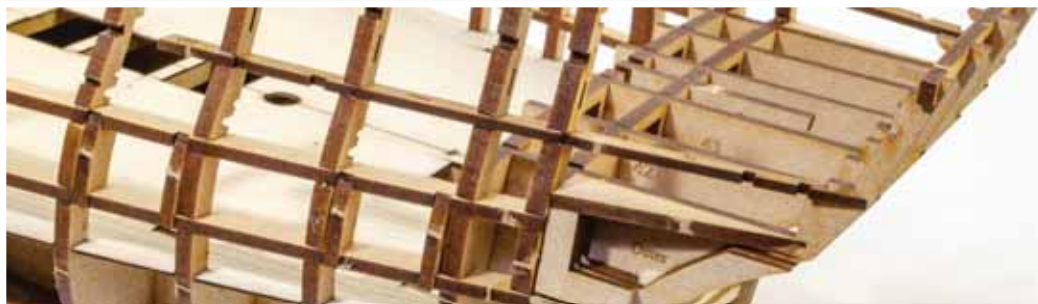
110. Glue these into the next set of bulkhead slots running from bulkhead #15 and terminating on the notches in the 'Outer' stern timbers.
