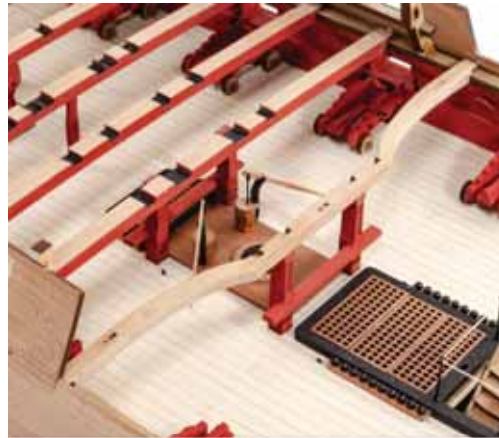
372. Glue the beam into place so that the engraved areas underneath will sit on top of the bits. Remove any red paint from the top of these first so you get good glue adhesion.
