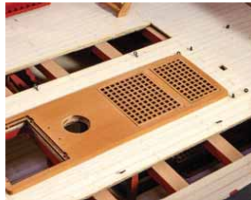
733. Glue the gratings into place. These are parts #410 and #411, found on the same 1mm wood sheet.
