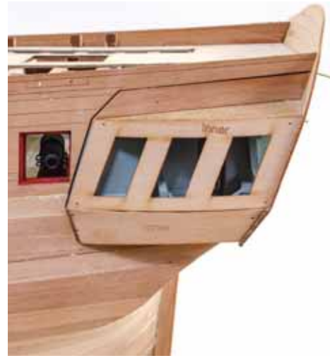
468. Now fit the lower part #568, bevelling the top edge so it sits up the previous part. You will need to trim this part to suit your own specific build.
