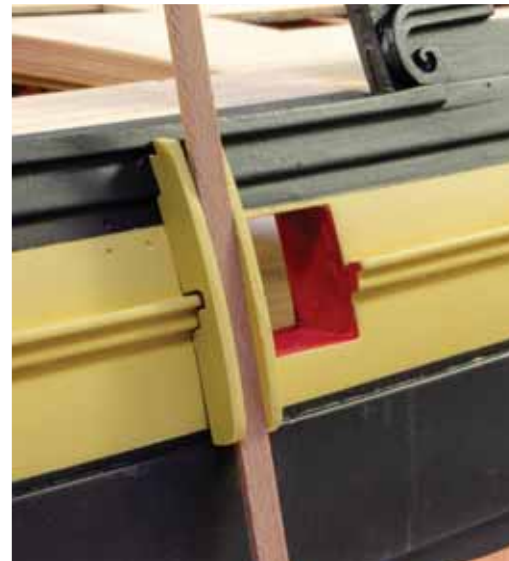
655. Use a piece of scrap 4mm plank as a spacer and glue the other #180 to the other side of the original one.
