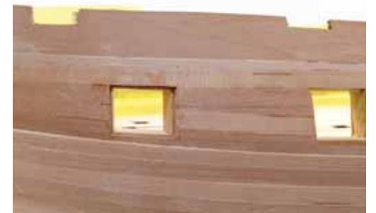
228. First fit parts #548 to the top and bottom of the forward most gun port. Now fit parts #547 to the vertical inner walls. All parts should lie about 1mm in from the front of the port, creating a recess. You will need to trim and adjust all gun port lining parts, for all ports.
