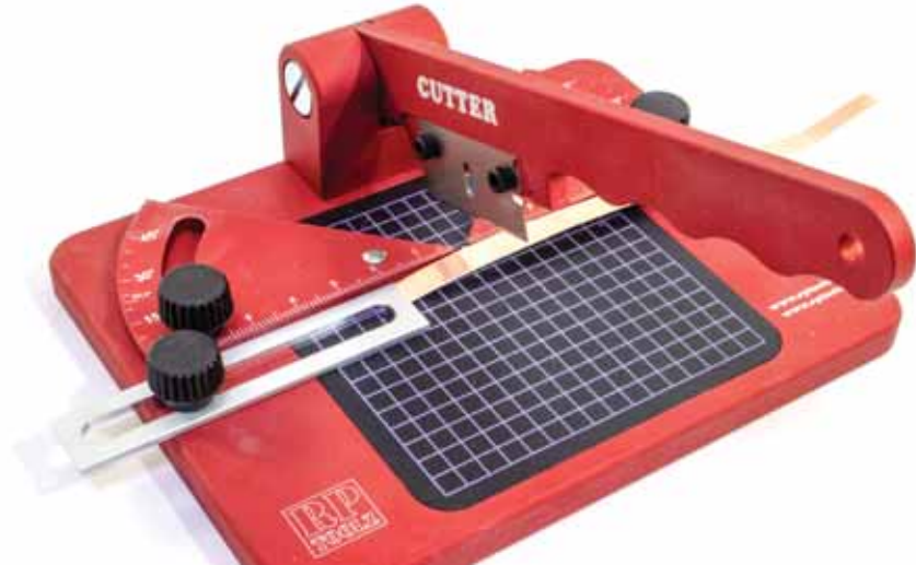
569. For coppering, we supply a roll of 6mm copper tape. This needs to be cut into pieces that are 18mm long. Save a few metres of the tape though. For cutting the tape into identical lengths, we used an RP Toolz mitre cutter due to the high quality. You can use a similar tool to make your plates. We estimate you will need around 2200 – 2400 plates.
