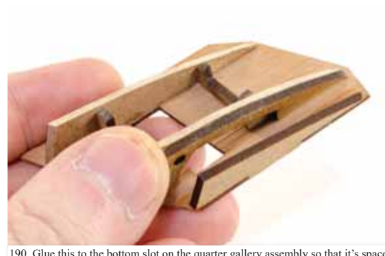
190. Glue this to the bottom slot on the quarter gallery assembly so that it's spaced evenly all along, in relation to the part you just glued into place. Leave to dry.
