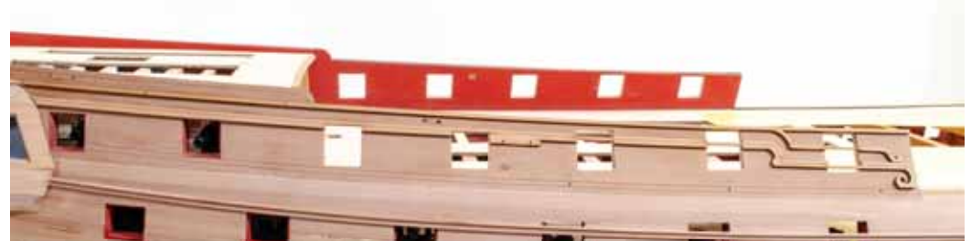
518. These must now be glued the upper areas of the outer bulwarks on both sides. The positions for these are easily seen as they are engraved for you.
