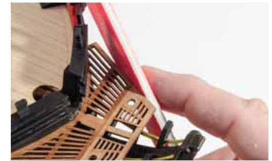
627. Take some sandpaper and sand flush any of the 'V' frames that protrude beyond the edges of the grates.
