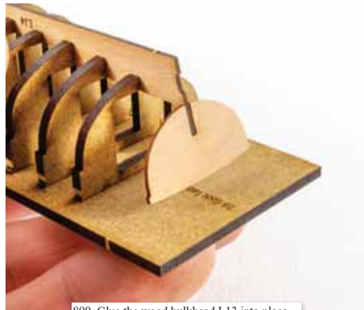
890. Glue the wood bulkhead L13 into place.
