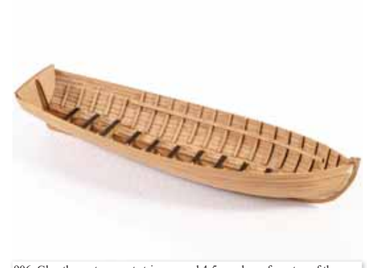
906. Glue the seat support strips around 4-5mm down from top of the bulwarks.
