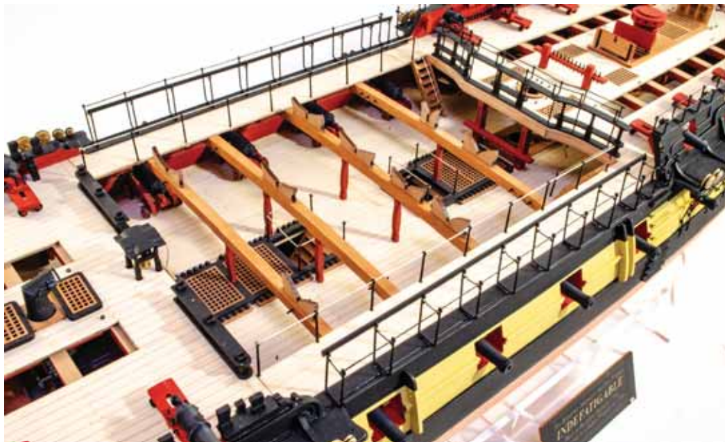
814. Here you see the rails alongside each of the waist gangways. The outer ones are rigged with 0.5mm black and a 188mm strip of 1mm x 2mm wood is used on the inboard area. 0.5mm natural rope is rigged along the inner stanchions and down by the side of the gangway steps.
