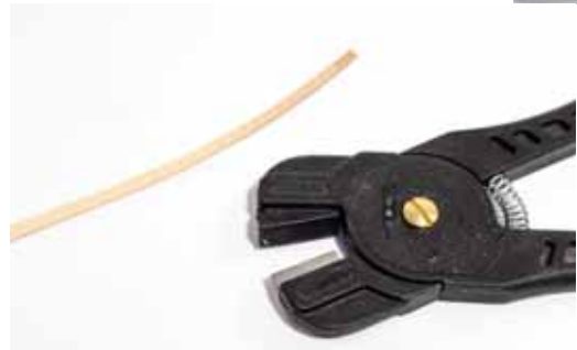
161. Again, a plank nipper is a great tool for helping form the curves in this 1.5mm lime. There's no need to soak to bend planks, and with any subsequent shrinkage that would occur.
