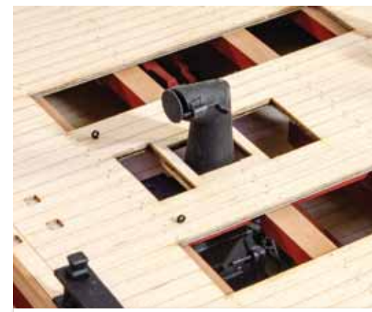
791. Glue the stove funnel into place through the deck, using CA glue. The funnel will point aft.
