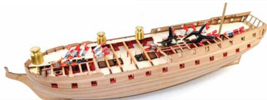
395. These are actually quite easy to fit, and unlike the lower deck, these can be installed as halved. Make sure you've removed char from the deck cutaways and exposed edges. Consider removing char from the bulkhead notches too. Another small tip is to use a jewellers file to slightly bevel the innermost edge of the notch, on the upper face. Test fit the part until you are happy with how this will progress. Also consider using some 8mm and 10mm dowel, slotted into the main and mizzen mast positions, to help with centring the part. Another tip is to mark the cut-outs onto the beams when you temporarily fit the deck. This will make sure you don't get glue in exposed areas. Now add glue to the deck beams etc. and fit the first half, clamping as you go. 2-inch clamps are great for clamping the cut-outs as the tail of them can also hold the opposite side down. Weight as you see fit and leave until dry.
