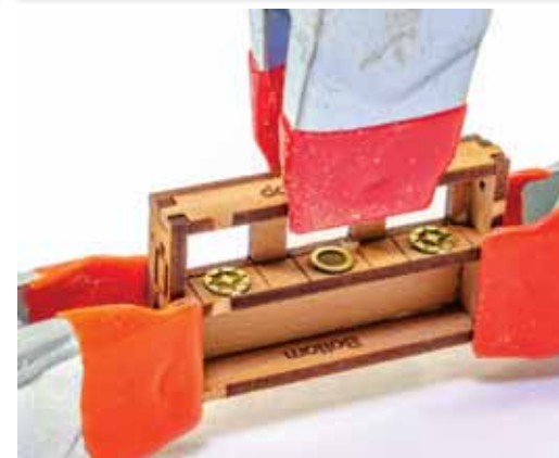
779. Take one of the front parts and glue/clamp into place. Make sure that it's flush all the way around.
