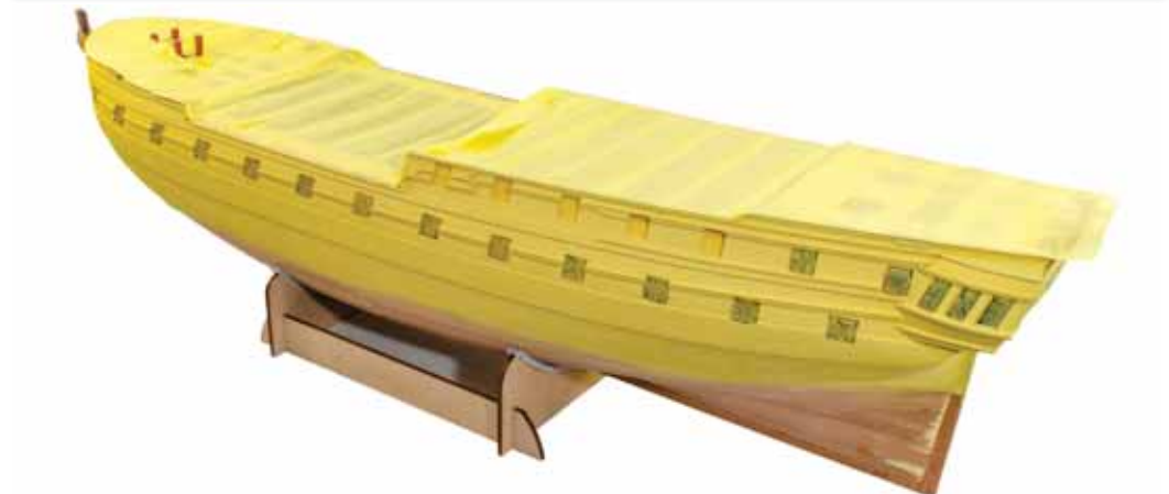
566. After carefully masking the hull and blanking any openings, paint the hull in yellow ochre. If you comprehensively mask any openings, you can airbrush this colour. Foam is used to stop paint getting into the gun ports. Note that all of the area to be painted is now in ochre. The reason is that the lighter paint makes it easy to see any defects in the hull at this stage. Paint using thin coats, run back and fill as necessary.
