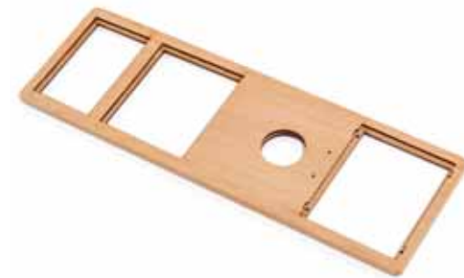
731. Clean up the part edges and apply clear varnish.
