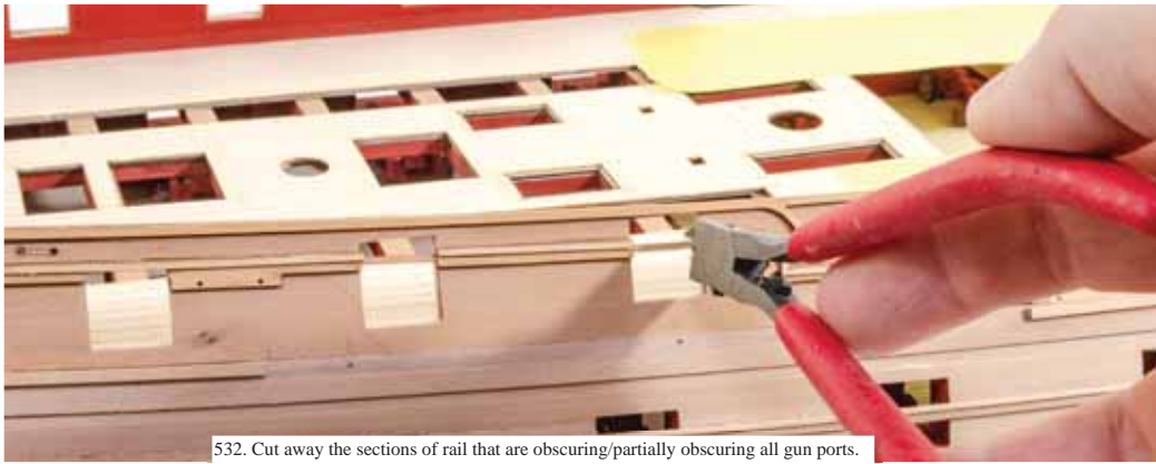
532. Cut away the sections of rail that are obscuring/partially obscuring all gun ports.
