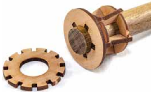
737. Glue that part into place as shown. From the 1.5mm wood sheet, now remove part #161.
