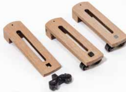
441. Glue the wheels into place as shown. You can then file down the resin on top so it's flush.
