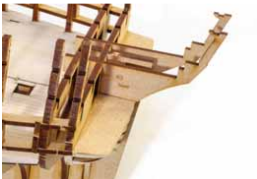
101. Take the pair labelled 'Inner' and glue them across the innermost slots in bulkheads #17 and #18, as shown. They will be flush with the top of those bulkheads and will lay flat on the stern section.
