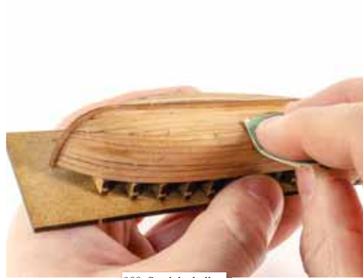
900. Sand the hull.
