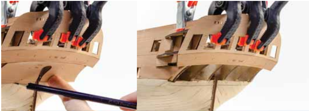
183. Sit the part on the hull, against the previous part #405, and push it into the stern curve. Use a pencil to draw a line along the bottom of this part, on the planking.
