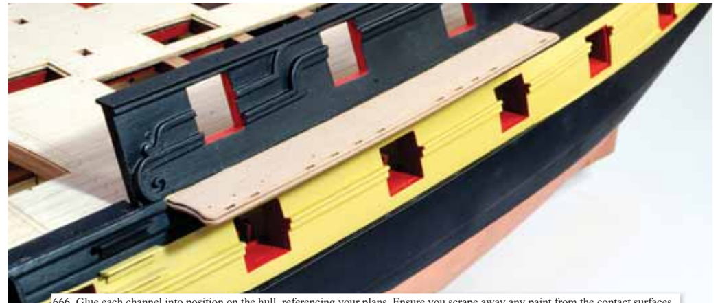
666. Glue each channel into position on the hull, referencing your plans. Ensure you scrape away any paint from the contact surfaces.
