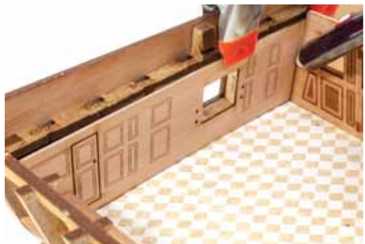
423. Temporarily clamp these in position as shown and then temporarily refit the rear screen, positioning it correctly. Draw a pencil line onto the side walls from inside the rear cabin, creating a point for masking before painting.
