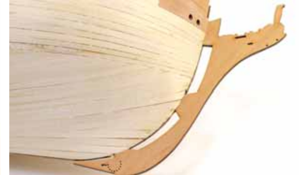
193. This can now be glued into position on the front of the hull. Do several test fits before you commit to glue. You may find a small rubber-tipped hobby hammer is useful for gently tapping this into place. Leave to thoroughly set.
