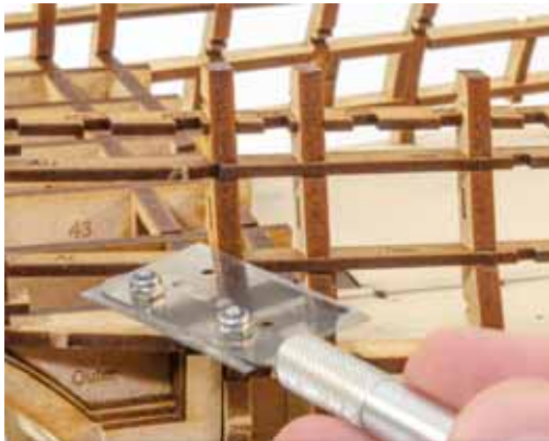
121. Carefully saw out this specific part of bulkhead #18 and file the area smooth. Also note that you can also saw and file away the parts of the strips that pass through the quarter gallery doorways.
