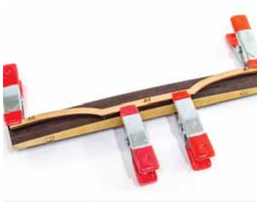
369. Add the alignment pegs to the three slots on the part, and then glue part #308 onto this. Clamp over the jig until dry.
