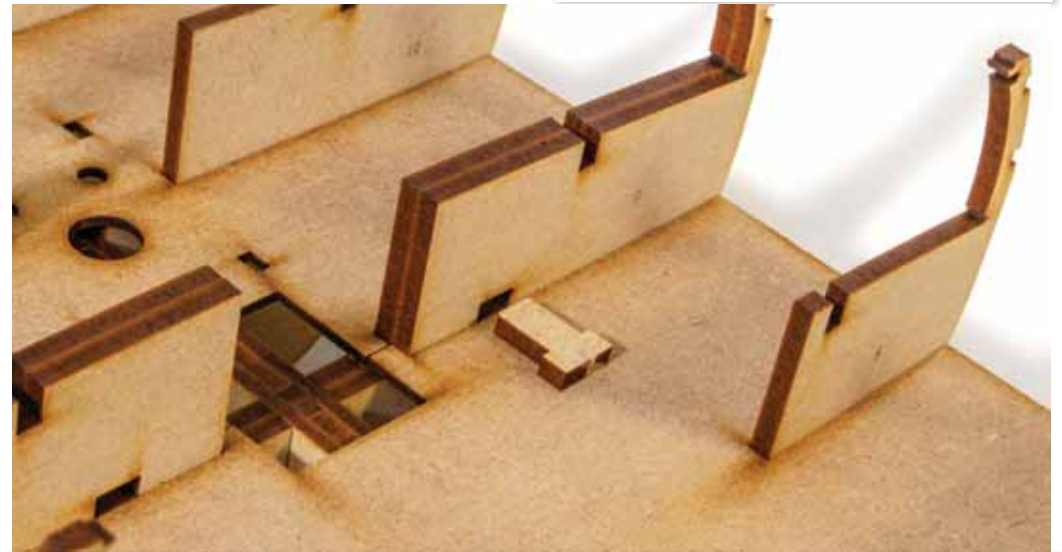
37. Also fit pegs K-3 into the slots that run through both bulkheads No's 9. On your model, these have moved outboard from where you see on this prototype.
