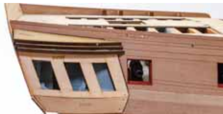
471. Sit (NO GLUE) the first one on top of the quarter gallery, pushed into the corner, against the stern. Now glue two more onto this, in the same way.
