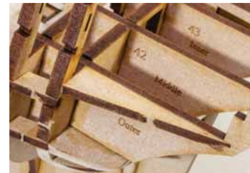
106. Here you see one of the parts in place, glued onto the 'Outer' stern timber that you just fitted, and against bulkhead 18. These are fitted so they are angled with the deck camber of bulkhead 18, and flush with the top of the 'Outer' stern timber. To achieve this you will need to slightly bevel the side which is glued against the 'Outer' stern timber.
