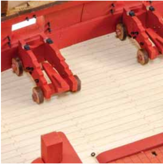
307. The carriages can now be plugged into the slots on the main gun deck, as shown. The wheels should sit flat on the deck.
