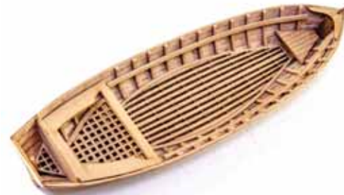
938. Now fit the seat support strips about 2 planks down from the top of the bulwarks.
