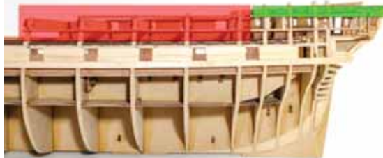
154. The larger side bulwarks can now be finally glued into place. IMPORTANT. This graphic shows a red area which will NOT be glued to the bulwark as these frames will eventually be removed later in construction. However, you can add a few tiny dots of glue in that area, just to tack the bulwark to shape during the build. NOTE: It is advised that you don't glue the area in green. This will later allow the upper bulwark to flex outwards to allow the poop deck bulwarks to be installed easily.
