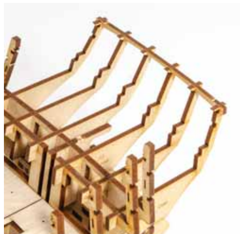
104. From the 3mm MDF sheet, remove part #45 and glue across the tops of the parts that you've just fitted.
