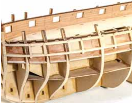
144. Here you see details of the sanding at both bow and stern. Note how there is almost zero char left on the bulkheads. If yours has char remaining, then you need to fair your hull more.
