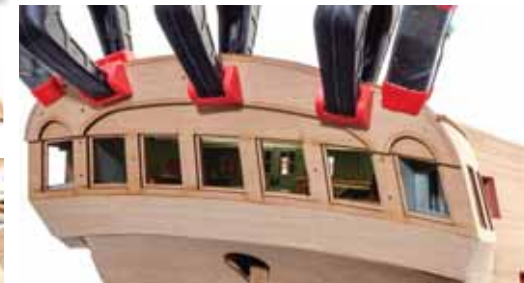
482. Carefully glue into position on the stern, using the engraved lines to guide you.
