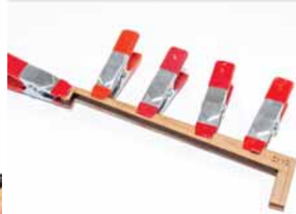
197. From the 4mm wood sheet, remove part #92. This is the stern/rudder post. From the 1mm wood sheet, remove parts #433 and #434. These are the external facings for the rudder post. Also remove two pegs #441 from the same sheet.
