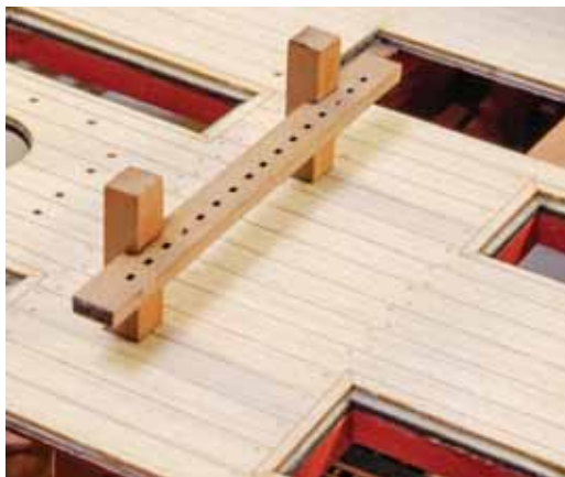
752. Glue the parts together as shown, while dry fitted to the quarterdeck. Paint the assembly in red.
