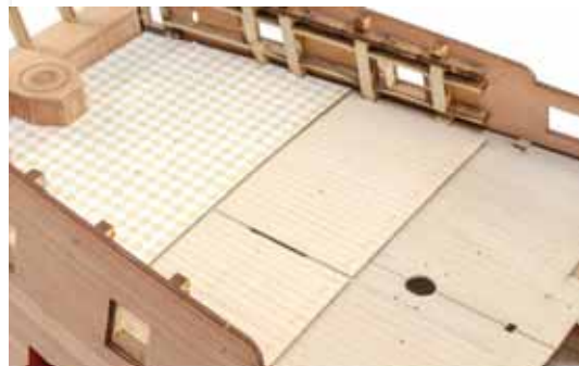
421. Whether you used the optional deck set or planked this with supplied materials, you now need to remove the rear screen and panel so this area can be worked on.
