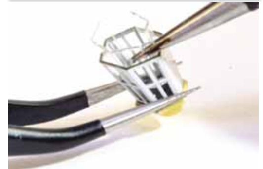
648. Remove the glazed parts from their sheet and bend into shape as shown. Push the glazing into the lantern.
