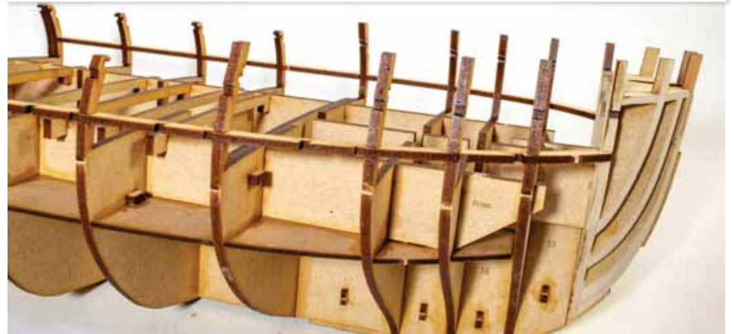
85. Fit each strip into the lowest row of bulkhead notches, stretching from bulkhead #1 thru to bulkhead #9. Ease the parts in gently. You can either glue these in straight away or fit them first and brush glue into the joints afterwards.
