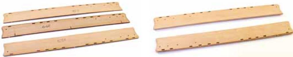
664. From the 0.8mm wood sheet, remove centre core parts #458. From the 0.6mm wood sheet, remove all outer panels #556. Round the outer edges of the inner core parts, and then round one side of the outer panels that sit onto the cores. Glue together as shown. Clamp as necessary. Make two.
