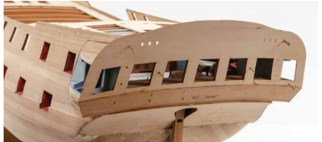
465. The counter and inner stern parts can now finally be glued into place, checking all the time that they are central to the hull. Note that there are some laser cut holes in the inner stern piece. These are there to help you temporarily pin the part while it dries. Also, the engraved side of this part must face inwards, towards the poop deck.
