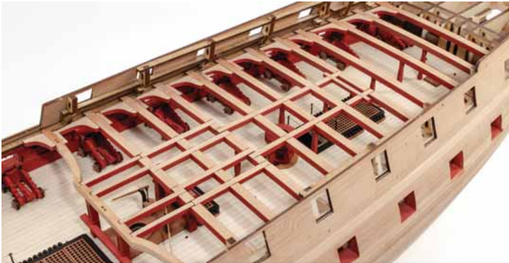
383. If you want to fit these parts (there is no requirement to do so), then please refer to the plan for positioning them. Here you see the knees in place, along with the horizontal lodging knees. If you wish to fit them, take your time in doing so.
