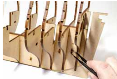
22. Glue pegs K-1 through the keel to lock bulkheads #15 and #16 permanently. You can now remove bulkhead #17 until a little later.
