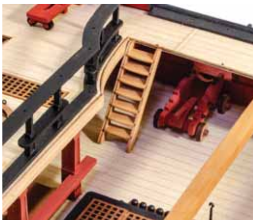
790. Using your plans as reference, glue the ladders into place as shown.
