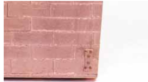
576. Fit these to the hull in the positions shown on the plan. You should be able to identify these areas through the thin copper tape, where the positions are engraved. Glue and pin these into position on both sides of the hull and paint the brass pins in a copper colour. Here you see the stern fishplate...
