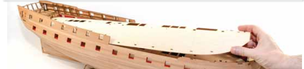
236. OPTIONAL: Test fit the deck to ensure a good fit. If necessary, sand the edges to make sure it lies down perfectly on top of the underlying ply deck. Apply glue to the ply deck area, ensuring that you have glue running around the various port openings etc. Then gently bend the maple deck and sit in in place, rubbing your fingers around the deck to make sure the glue is squeezed around the connection and the deck lays flat.
