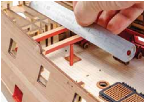
362. As the pillars will have to be height adjusted, it is VITAL that you run a straight edge over the beams and check they aren't at different heights to those around them.
