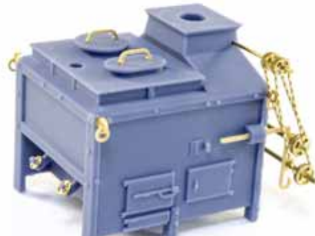
348. Slide another BS-4 onto the thin brass rod, and a BS-5 onto the thicker brass rod. Move the chain inwards but not to it touches the smaller chain. Now use spots of CA to lock everything in position. Trim the brass rods so they protrude just a little more than the chain assemblies.
