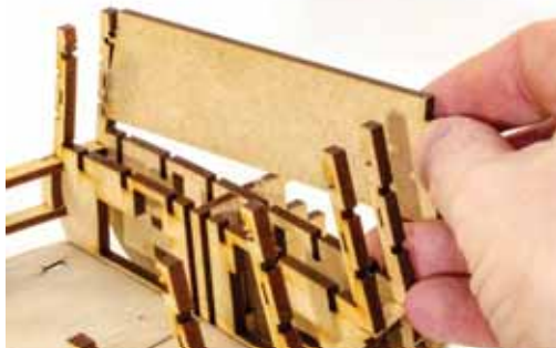
99. Carefully remove the plank panel from bulkhead #18. You can do this by gently twisting at the part and pushing in either direction while supporting the bulkhead ears. That panel can now be discarded.
