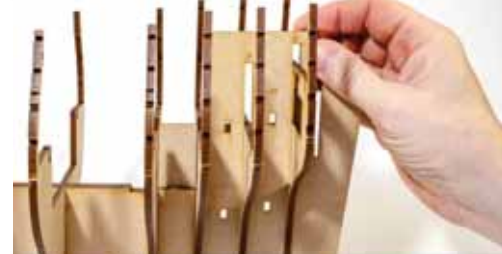
21. As with the previous parts, slot one of these on either side of the keel, holding bulkheads #15 and #16 into position. Bulkhead #17 is only there at the moment to ensure correct positioning of the current parts.
