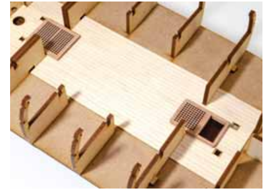
44. These hatchways can now be glued into place on your ply/maple deck as shown.
