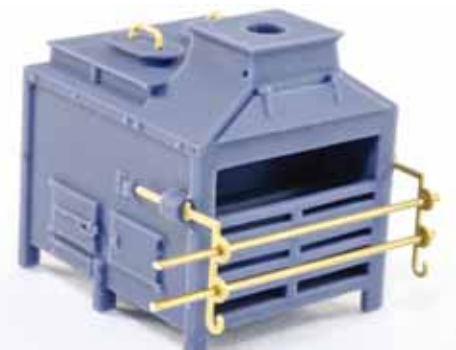
340. Cut two lengths of 0.8mm brass rod as seen here, and glue into place. You can cut these slightly overlong on the left of the stove as they can be trimmed to length after.
