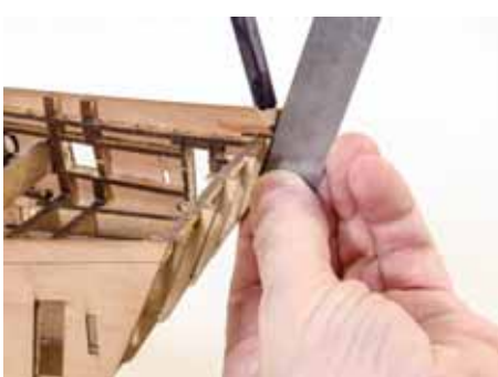
165. It will have been apparent that the side bulwarks protrude slightly at the stern. This is normal as we've left a small amount of timber to cater to variations in the hull. These are now marked in alignment with the stern, using a steel rule and pencil.
