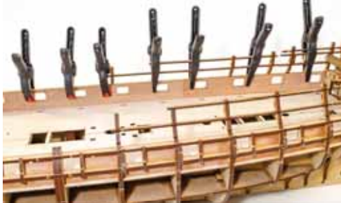
132. Again, soak if necessary and allow 24hrs to dry out before clamping to the hull and painting glue into the joints from the rear. When set, repeat the process with all bulwark sections on the opposite side of the hull.
