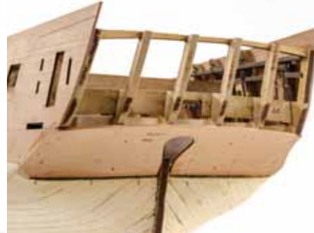
185. You can now remove the narrow counter and upper stern face. Those can be put away until later in the build.
