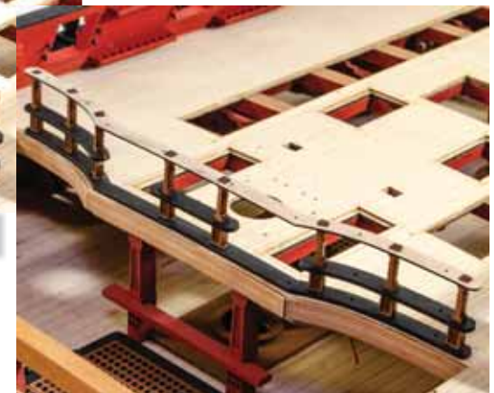
688. Now glue part #499 to the top of the pillars. If any of the columns protrude, then sand flush with top of part.
