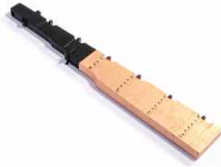
588. Add brass pins to all of the rudder straps and paint in black/copper accordingly.
