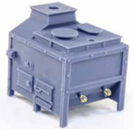
338. Glue two parts BS-8 to the rear of the stove as shown. You may need to slightly drill these out.
