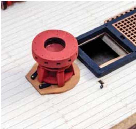
319. The capstan assembly can now be painted red and fitted to the deck as shown. Make sure the dowel is pushed fully into the hull and into the deck below. You can now finally glue the pawls into place, noting the orientation of the capstan in the photo.
