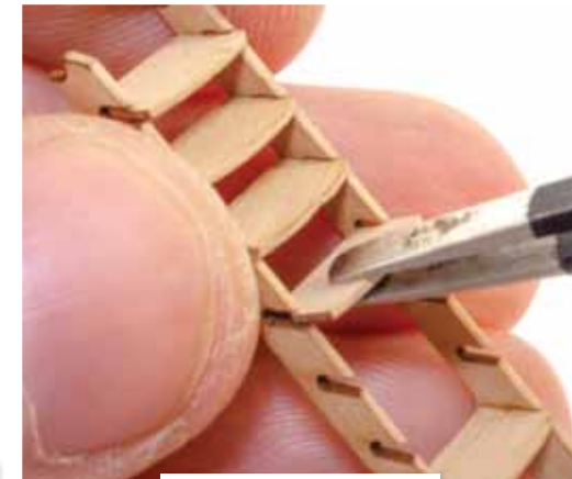
787. Now fit all the remaining steps.
