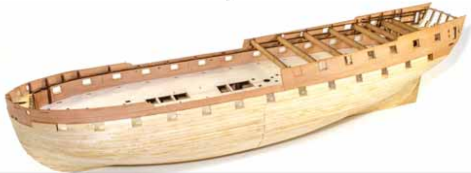
163. You will possibly have your own way of planking, and that is fine. This kit is designed for advanced builders. On the prototype, we've planked this simply. As I plank downwards, it becomes a little more difficult for the planks to lap flat against the bulkheads. At this point, I decided to then start planking at the bottom of the keel and progress upwards towards the planks I previously added. Note how I've left the planks short of the keel back edge at the stern. This will make it easier to taper the planks into the MDF.
