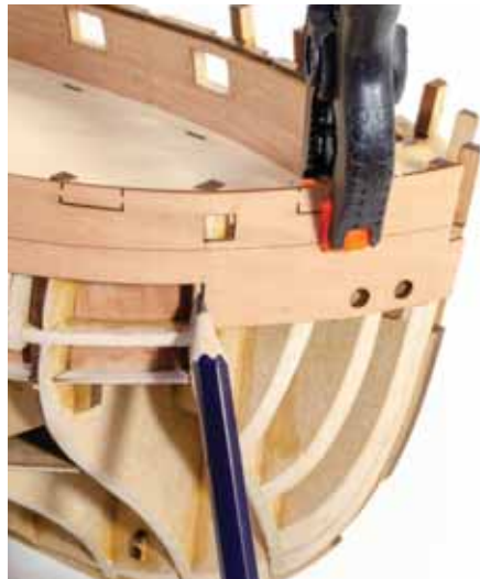
146. Clamp these into place on the hull (DO NOT GLUE). You may find it necessary to soak these parts for 30 minutes in warm water. If you do this, you MUST leave the parts for 24hrs to dry and to shrink to normal size again as pear expands a lot when wet. Note that the main bottom edge of this part lies along the top of the fore gun port frames.
