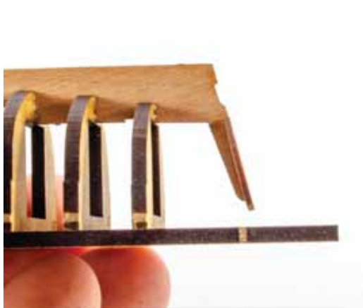
891. The angle of this part will match the angle of the rear keel.
