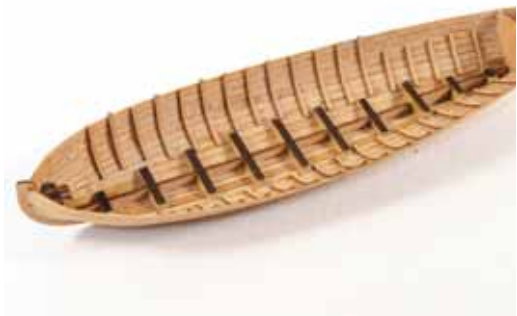
870. And fit out the hull with ribs, using 5mm spacing.
