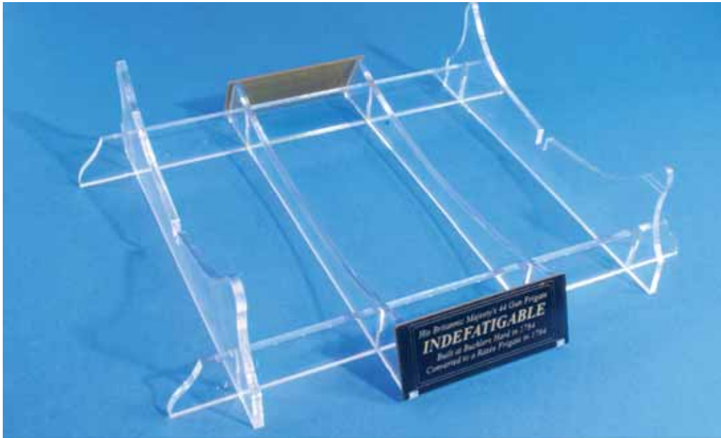
946. The acrylic cradle now needs to be built. This is very self-explanatory. When built, add the name plates. No glue should be needed for the cradle.
