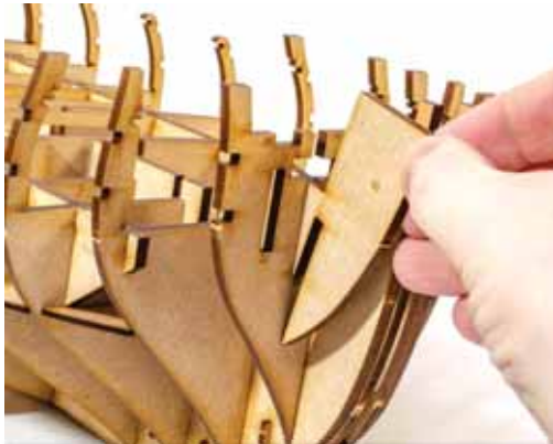
67. Now glue parts #20 into place on bulkhead #1. This will hook over bulkhead #2, but don't glue it to that bulkhead yet.
