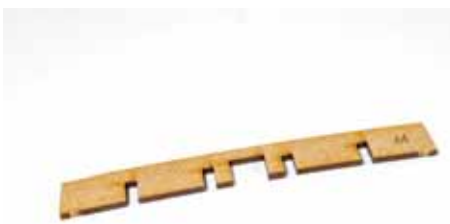
165. It will have been apparent that the side bulwarks protrude slightly at the stern. This is normal as we've left a small amount of timber to cater to variations in the hull. These are now marked in alignment with the stern, using a steel rule and pencil.
