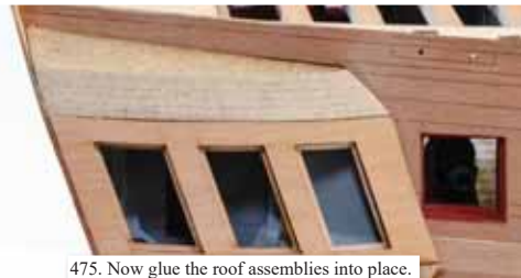
475. Now glue the roof assemblies into place.
