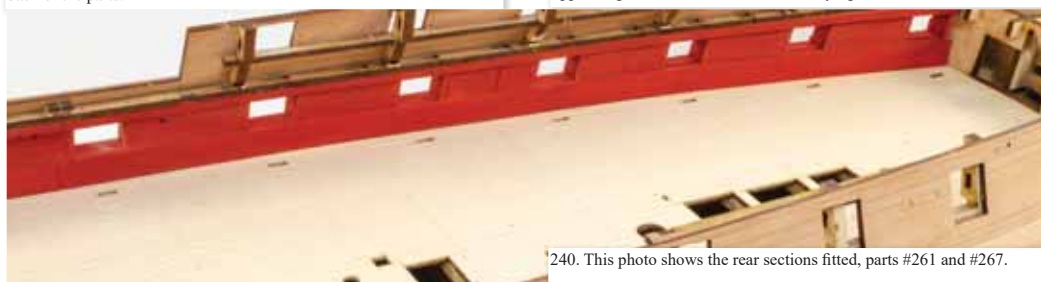
238. From the 1mm wood sheet, remove parts #260 and #261, and parts #266 and #267. These are the spirketting which runs under the gun ports, and the upper ledge which runs above the ports. Each section which runs full length of the inner bulwark, is split into two parts each for ease of fitting. NOTE: On the parts sheet, there is an 'F' and 'R' engraved onto the sheet. These indicate the foremost point of both the upper and lower, and the rearmost point. Write these idents onto the back of the parts.
