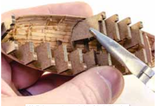
930. Twist away the remainder of the bulkheads.
