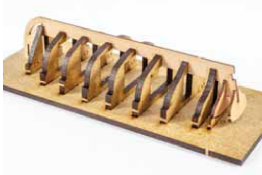
824. Glue the keel into the slots in each bulkhead. When dry, glue bulkhead C15 into place, from the 1mm wood sheet.
