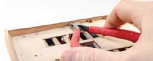
484. Use cutters to remove all the MDF bulkhead ears above deck level. Do this on all decks.
