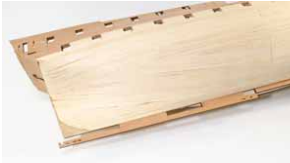
196. Now glue part #91 into place, and also to the part #90 that you just fitted. Ensure parts #90 and #91 are perfectly in line with each other. Clamp as necessary.
