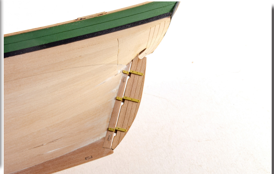
124. Glue the rudder to the hull. From the PE sheet, attach hinge parts #PE-23 to the rudder post as shown.
