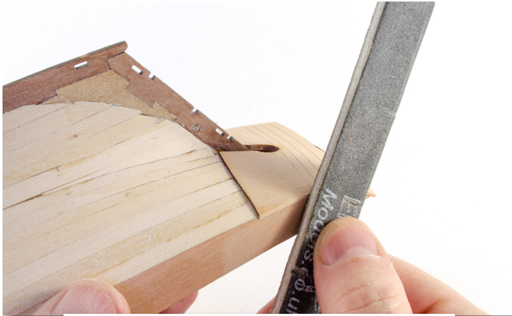
73. Once set, sand the overhang of this part so that it's flush with the bulwark.
