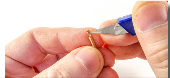
110. Remove part #55 from the 1.5mm wood sheet. This will fit inside the stern, but you'll first need to bevel the inside slots so the part sits more or less horizontal to the slope of the deck.
