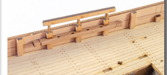
104. Now remove the two parts #46 from the same 2mm wood sheet. Note these are labelled as 'AFT'. Glue these into place across the rear sets of timberheads, as shown.
