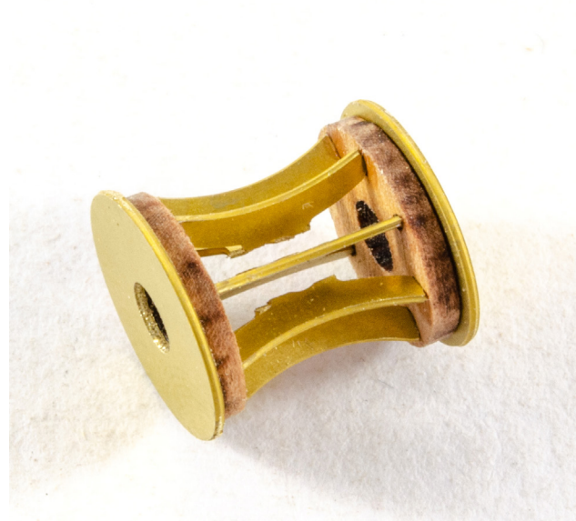
172. Glue these to either side of the assembly. You can then remove the dowel.
