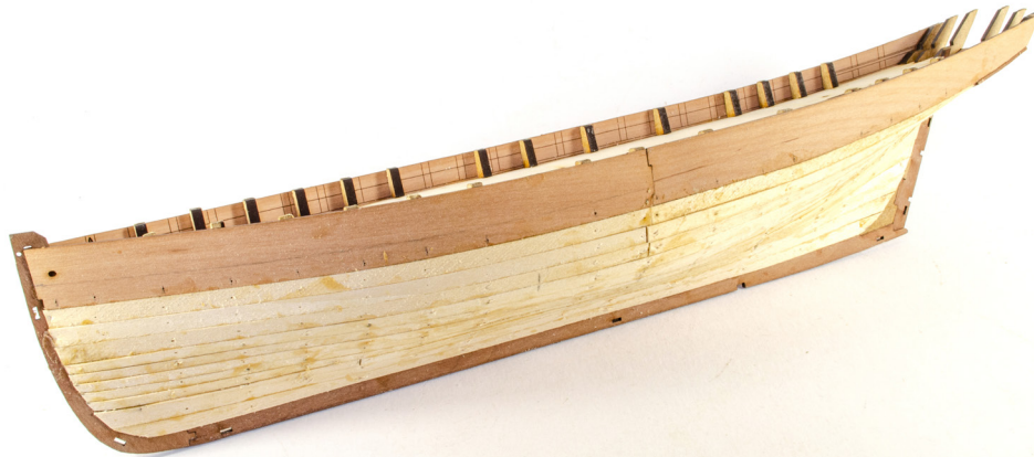
66. Work your way downwards in the same way. You may get to a point where you want to work upwards from the keel. That's perfectly ok. Plank the hull until complete. If there are gaps, add small pieces of wood to fit in them. Those are called 'stealers'. Note how the planks at the stern create a curve. That's so the outer keel face can eventually be added. If you are unsure, please look at the photos which proceed this one.
