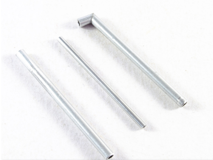
201. CHIMNEYS: Use the 2mm and 3mm alloy tubes to make up three chimneys as shown. One of these will need bevelling at the top and a short, bevelled section fitted with CA. Check plans for dimensions.
