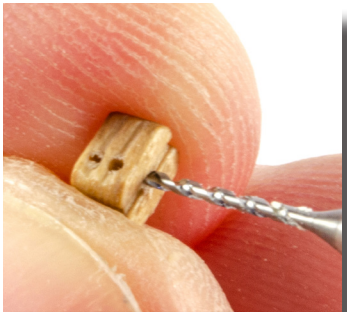
163. Take a 4mm double block (#F-14) and drill a 0.8mm hole right through the middle.
