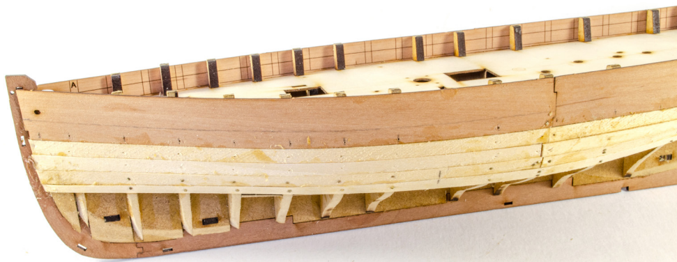
65. The tapered plank can now be glued and pinned as shown.
