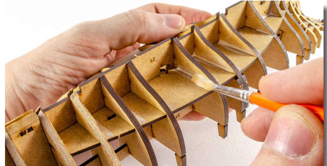
40. Now we can finally glue things together. As this model has many slots, this is the way we recommend applying glue for the main structure. Use white glue or Titebond, slightly diluted, and paint this into the various joints that make up the skeleton of Erycina. Make sure all parts are fully in position as you are doing this. When the glue is applied, leave to thoroughly set.
