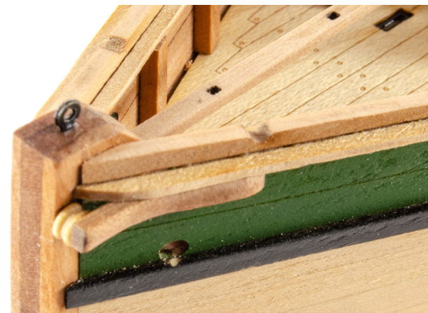
209. Glue parts #93 into place as shown, on the engraved marks on the gunwale. Also note that the Bow Roller has been fitted. Glue #47 into position using plan as reference. Now use the short length of 1mm brass wire which is long enough to fit through hole in prow and rest up against the part you just fitted. The brass wire needs to be flush with other side of prow. Fit the wire, trapping the 2.5mm thimble between the prow and the knee.
