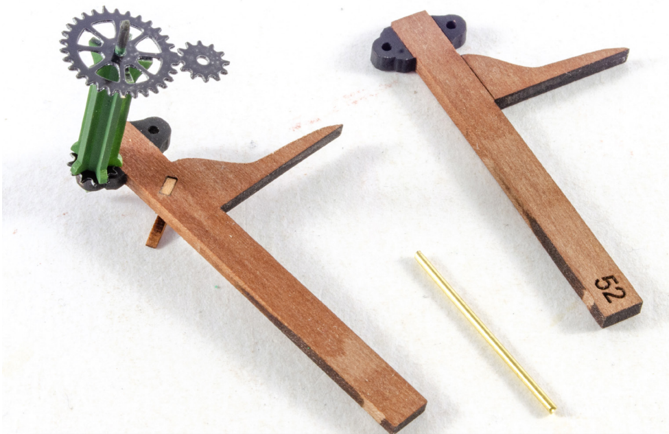
193. Follow the illustrations on the plan sheet and assemble the main windlass as shown here.
