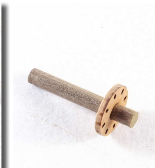
169. Slot, don't glue, one of the discs onto the dowel.
