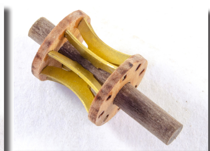
170. Now slot the other disc onto the other end and then sit the PE parts into the holes between the two, ensuring the holes are aligned on both discs. When you have all PE fitted, push the discs so the PE is properly trapped between them. Twist and adjust as necessary. Use a little CA on a cocktail stick and apply it to all joints.
