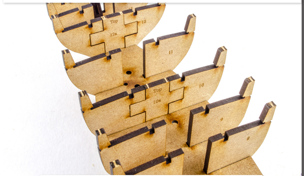
28. Now glue parts 10a and 12a into position on their respective bulkheads.
