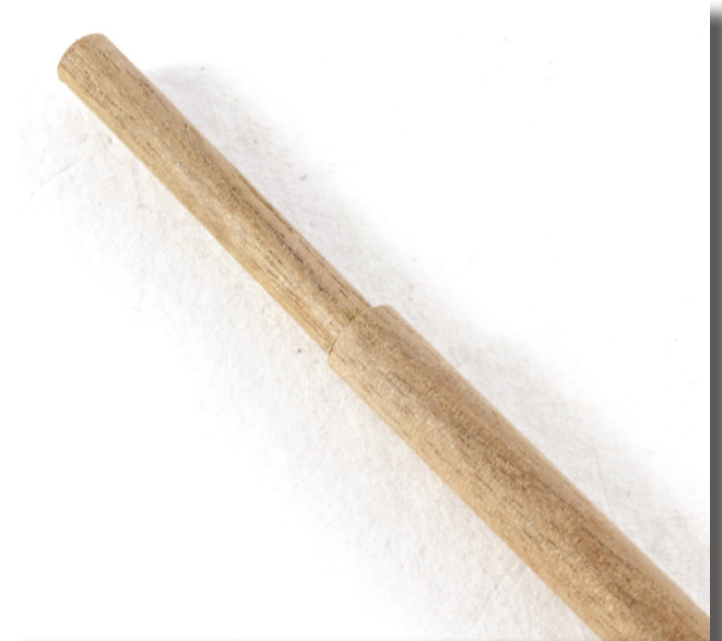
214. FOREMAST: Take the lower section of the foremast and reduce in diameter around the top area, as shown on the plan.
