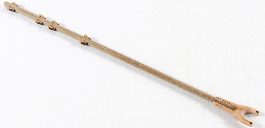
225. Bevel the jaws as previously. This is very important as you want to be able to angle the gaff to accommodate the correct angle. This is especially important if you are fitting sails.
