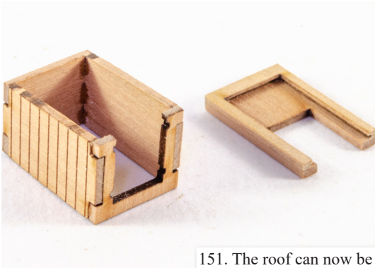
151. The roof can now be glued to the companionway. From the 0.6mm wood sheet, remove part #114a.
