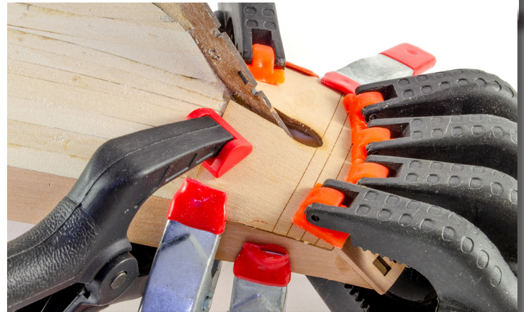
72. We found this part didn't need to be soaked before fitted. Glue into position and make sure it's clamped around the edges and in the concave area on the hull underside.
