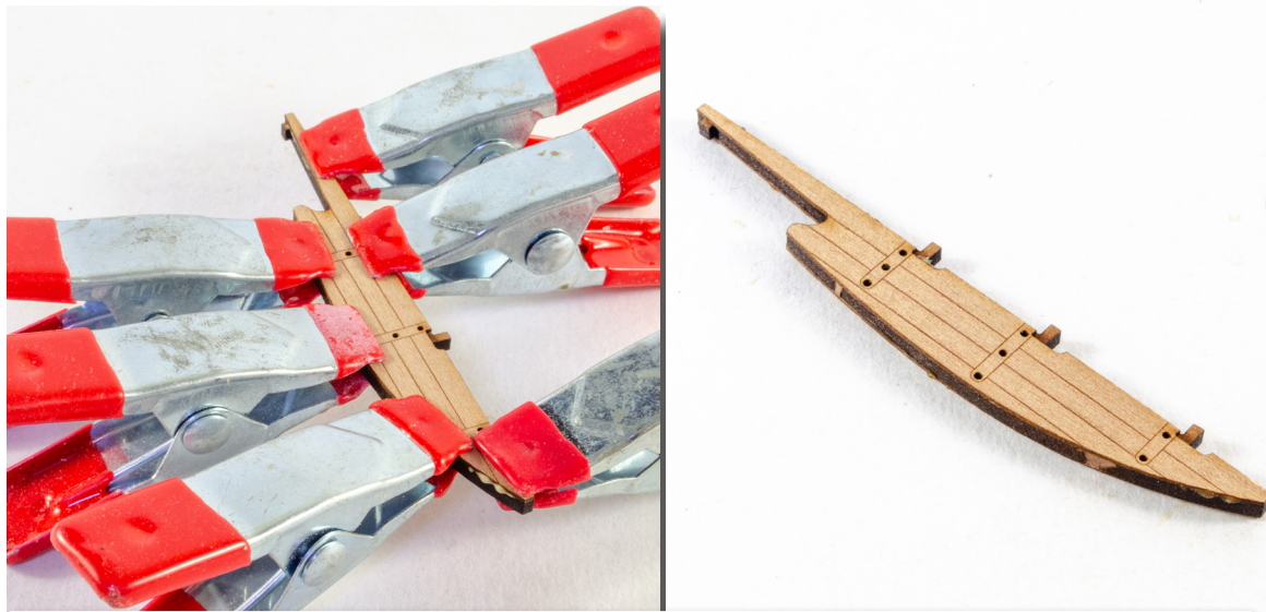
122. Glue the thin outer parts to the inner 2mm rudder, with the engraved faces outwards. NOTE: Apply glue to the 2mm part so as not to curl the thinner timber. Make sure everything is properly aligned and then clamp until dry.
