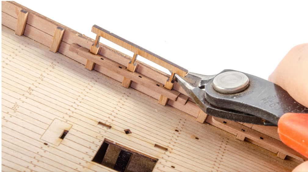
107. Use a pair of cutters to snip the cross bar and connector from the top of the joined timberheads.
