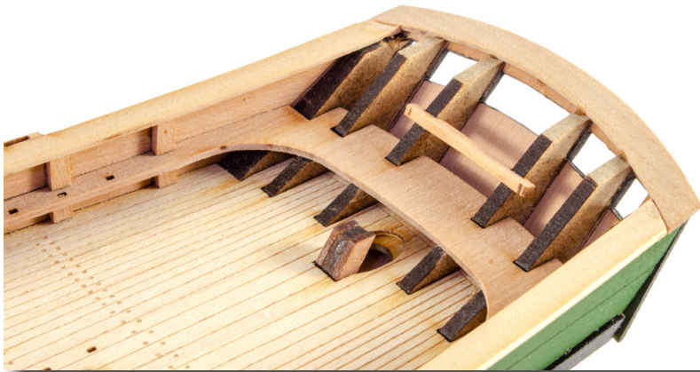
118. This is now glued into place as shown. Sand any overhang at the sides, flush with the rails you previously fitted.
