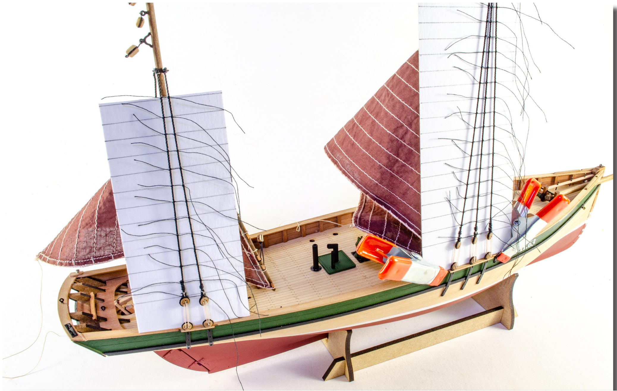
234. STANDING RIGGING: You now need to add the standing rig. The main part of this are the shrouds and ratlines. These are a bit of a chore, but on a model this size, they don't take too long. You need to do this on the model. There is no way around this. You just need a couple of pairs of tweezers and some patience. Use dilute PVA to sieze the knots and trim then close to the lines when complete. To help with ratline spacings, we have included a template on the plans. Cut it out and paste to some card. Do the larger shrouds first, then you can trim the template to fit the mizzen shrouds.
