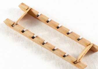
140. Glue the other side into position and make sure nothing is twisted. Leave to dry.
