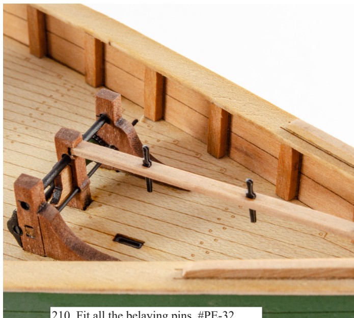
210. Fit all the belying pins, #PE-32.
