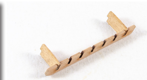
139. Glue a step into the top and bottom slots in ladder side. Leave to dry.
