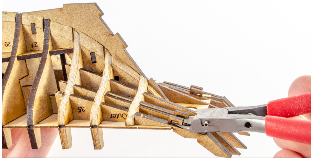
47. As everything is now securely glued, the 'safety gates' on the middle and outer stern parts, can now be snipped off flush with the part.
